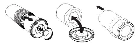
Unscrew bottom cover and remove plastic bag from filter.
