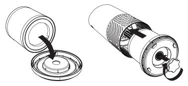
Secure filter on bottom cover and replace inside the purifier.
