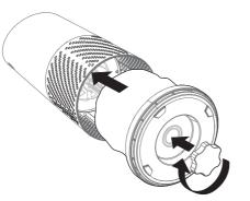
Secure filter on bottom cover, slide both into purifier, and reattach knob.
