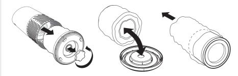
Unscrew knob, loosen bottom cover, and remove plastic bag from filter.
